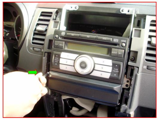
5: Remove the power connectors of console
