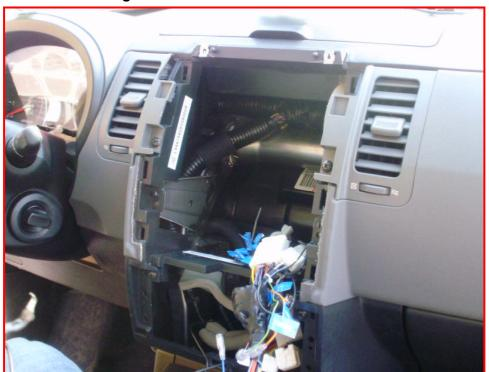
7: Connect the original cables to FLYAUDIO's cables
