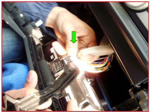
6: Remove the power connectors of original main unit
